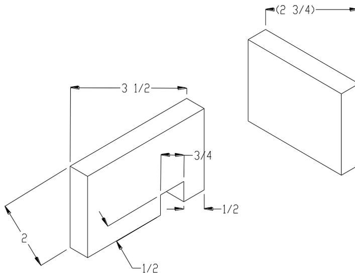
2. Screw the Mitre Slot Base with 2-drywall screws to the main board as shown in drawing.
